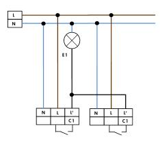
Standard mode with 1-channel motion detector with permanent light function
