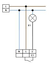
Parallel connection with 1-channel motion detectors
