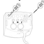
Mount the plug-in socket with two screws and the enclosed seal rings on a firm base. (Pay attention to inserting of the connection cable, see point 3)
