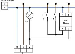
Standard mode with 1-channel motion detector with NC pushbutton
